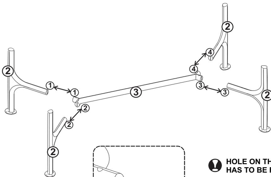
**!** HOLE ON THE LEG STRETCHER HAS TO BE FACED UPWARD
